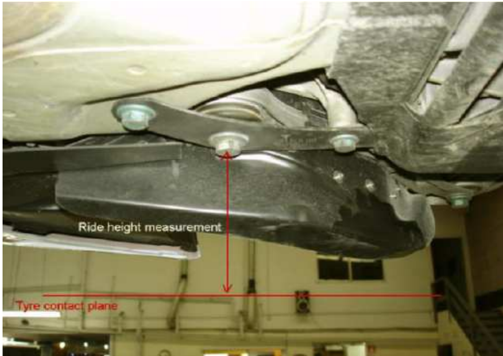
RIDE HEIGHT MEASURING POINT - FRONT AXLE TYPE 996
